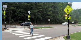
Rectangular Rapid Flashing Beacon (RRFB)
