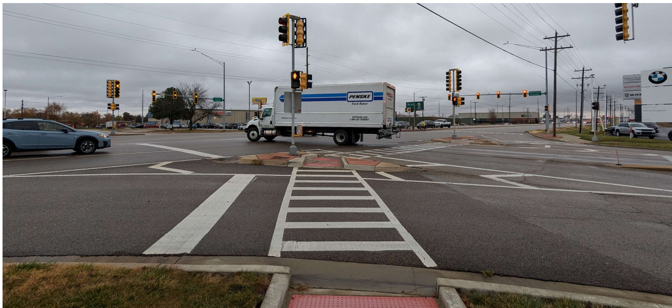
A typical multi-stage pedestrian crosswalk design.
