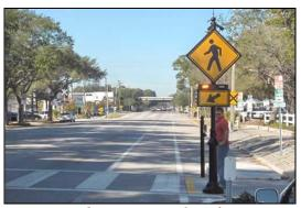
Figure 4.7. Left – median refuge island (courtesy Pedestrian Bicycle Information Center). Right – Rapid Rectangular Flashing Beacon (courtesy FHWA).
